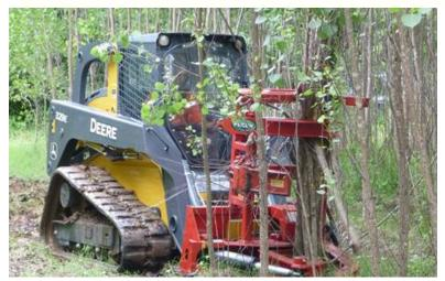
Non-traditional equipment is tested for harvesting small trees as an energy crop. The red attachment is a sheer felling head, and allows the skidsteer to accumulate several small stems at a time. Photo by Dana Mitchell, U.S. Forest Service.
